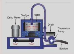
The Lubricant to be cleaned is passed through a rotor, driven by Electric Motor. Centrifugal force 2000 times gravity is exerted on the particles, depositing them on inner wall of rotor as dense cake. Clean oil returns back to the oil tank.
